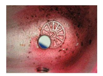
NOTE: the hole on the production date punch, as shown, still allows you to read the production date
